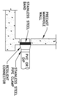
STANDARD PRECAST MANHOLE PIPE CONNECTION
